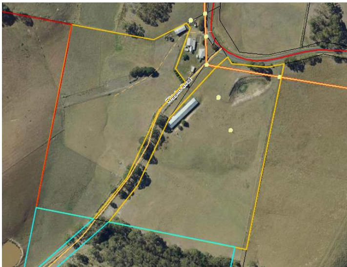
Figure 6: High voltage transmission line (orange line) running along inside the front boundary of CT 121549/2, and power poles leading into the lot (yellow dots).
