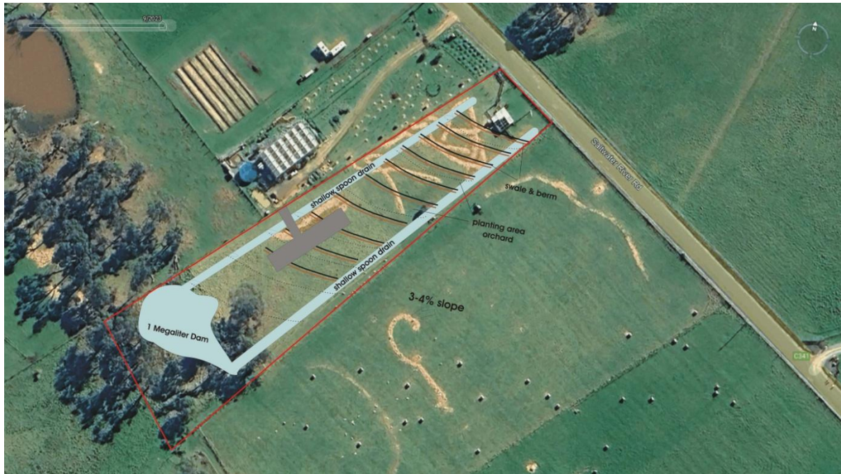
Image 2: Site layout with contour planting and water management including dam site
